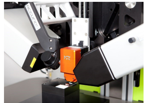
NaniteAFM integrated in the Accurion nanofilm_ep4 imaging ellipsometer
