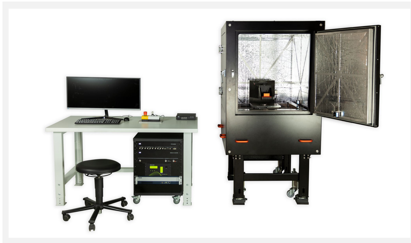
Figure 2: Alphacen tip scanning AFM, with a motorized stage providing full access to 300 x 300 mm 2 large samples with weights up to 40 kg. The system is placed in an acoustic enclosure and includes active vibration isolation to reduce the effect of environmental disturbances.
